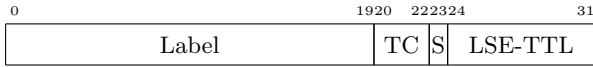
Figure 1: The MPLS label stack entry (LSE) format. An LSE is made of four fields, the label , the traffic class , the bottom of the stack , and the time-to-live .
