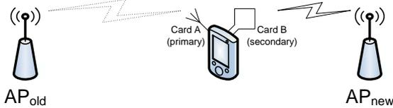
Figure 2: Multi-radio handoff scenario in MultiScan.
