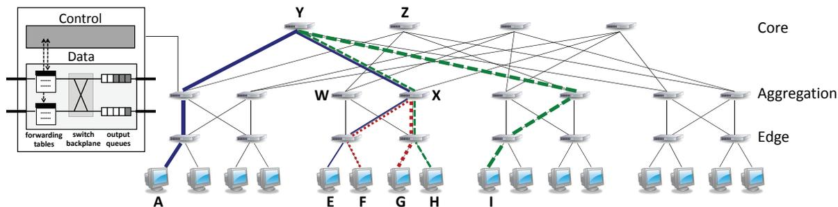
**Figure 2: A FatTree network with 4-port switches. VL2 is a variation on this topology. End hosts A, G, I simultaneously transmit to E, F, H and collide at switches Y and X, but there is sufficient capacity to route all flows at full rate.**
