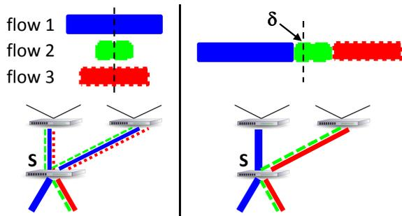
**Figure 1:** A set of flows to the same destination arrives at switch S. PacketScatter (left) splits every flow, whereas LocalFlow (right) distributes the aggregate flow, and only splits an individual flow if the load imbalance exceeds  $\delta$ .
