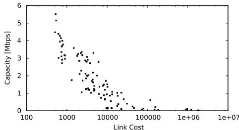
Figure 1: X-UTT (x-axis) relation to link capacity (y-axis).
