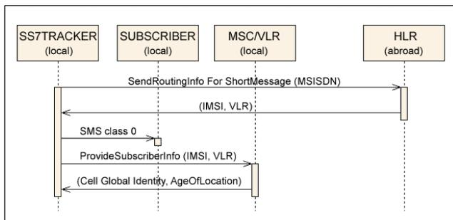
Figure 2: Messageflow for obtaining location of an inroamer
