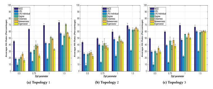
Figure 4: Hit rate comparison by varying Zipf parameter (cache size=100 MB) for centrality-based (NICE, Degree, Closeness, Betweenness, Eigenvector), non-centrality based or social-unaware (LRU) and non-collaborative (LRU-Individual) caching.
