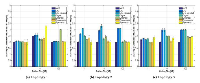
Figure 5: Hop count comparison by varying cache size (Zipf parameter=1) for centrality-based (NICE, Degree, Closeness, Betweenness, Eigenvector), non-centrality based or social-unaware (LRU) and non-collaborative (LRU-Individual) caching.
