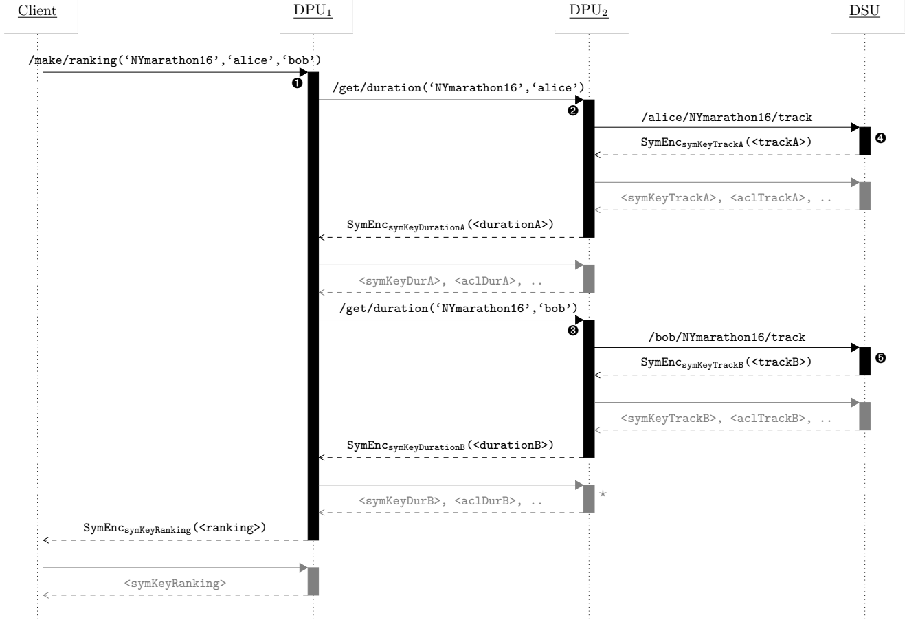
Figure 2: Computation Chain: ❶ Client requests ranking from NY Marathon 2016 including Alice and Bob ❷❸ Triggering computation of Alice’s and Bob’s duration (intermediate results) ❹❺ Requesting the time-location tracks of Alice and Bob on which all computations are directly or indirectly based * Further details in Figure 3: Fetching ACLs and keys for each step are just foreshadowed in this Figure.
