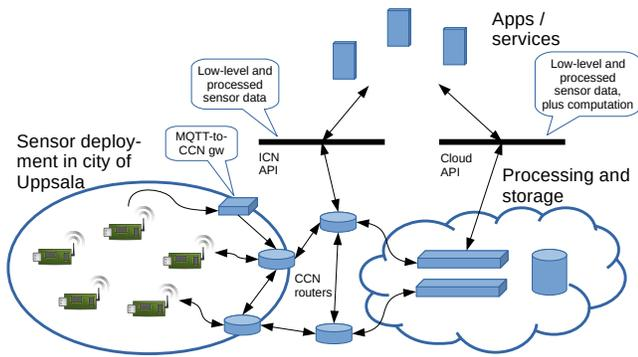
Figure 1: Uppsala city IoT testbed with ICN transport
