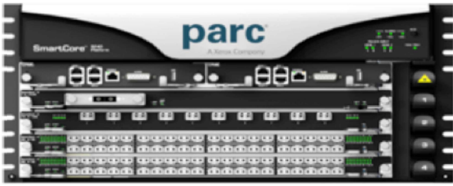
Figure 2. PARC Router Platform
